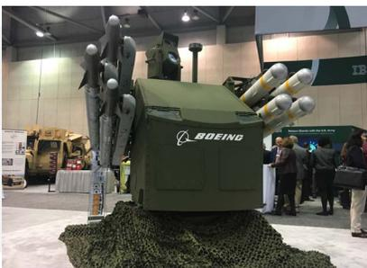
**Boeing Old Avenger is a blast from the past.** The company modernized the Avenger air defense systems—originating in the 80's—to fill the Army's need for Short-range Air defense (SHORAD) Gap. The Avenger will be upgraded to perform like a multi-mission launcher. [More here >>](#)
